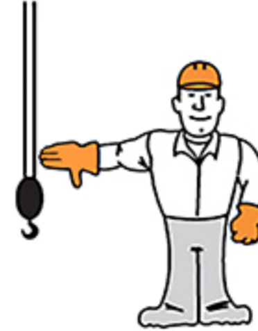
Lower the Boom Raise the Load
