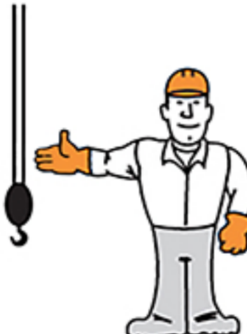
Raise the Boom Lower the Load
