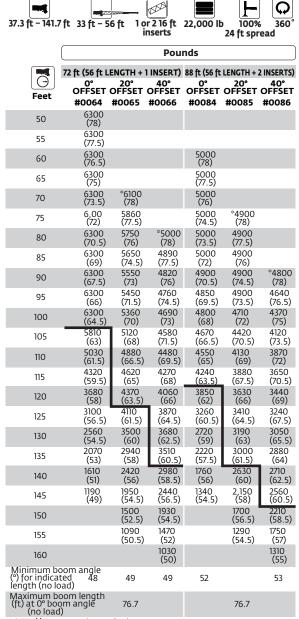
NOTE: () Boom angles are in degrees. A6-829-103478 #LMI operating code. Refer to LMI manual for operating instructions. \*This capacity is based upon maximum boom angle.
