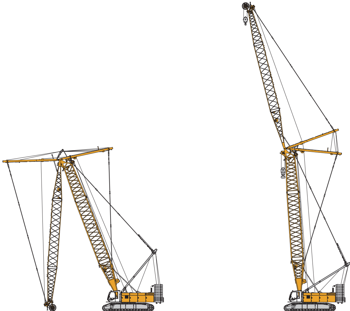
Erecting of main boom and luffing jib
