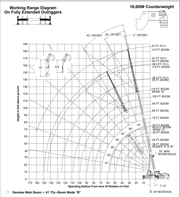
Note: Boom and fly geometry shown are for unloaded condition and crane standing level on firm supporting surface. Boom deflection, subsequent radius, and boom angle change must be accounted for when applying load to hook.
