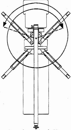
Pioneer Cranes utilizes the "X" outrigger design and goes one step further. Instead of just 375 degrees of rotation, Pioneer gives the operator a full 500 degree boom rotation. This truly allows working over the front of the unit with <u>no</u> compromise. Compared to other manufacturers, Pioneer gives you full stability and total access to the job site, It's a tough combination to beat.
