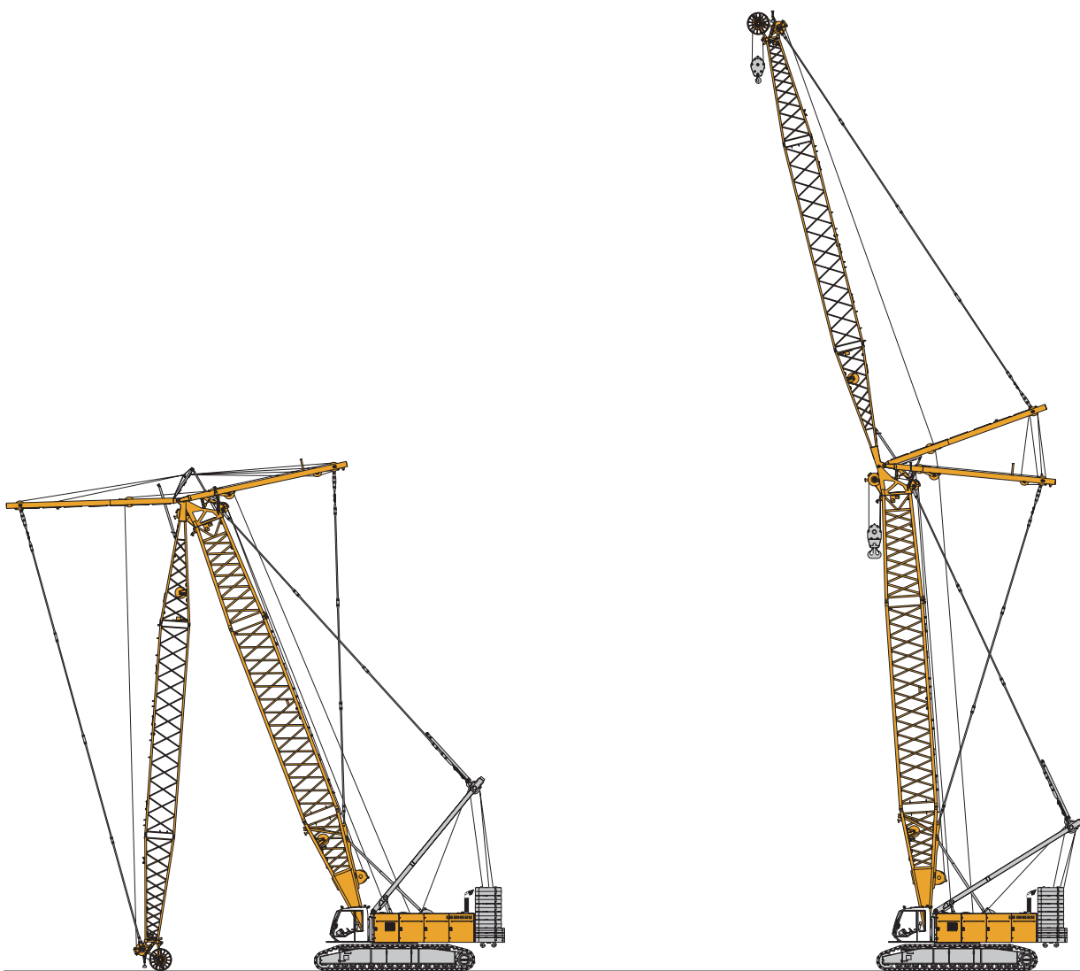
Erecting of main boom and luffing jib
