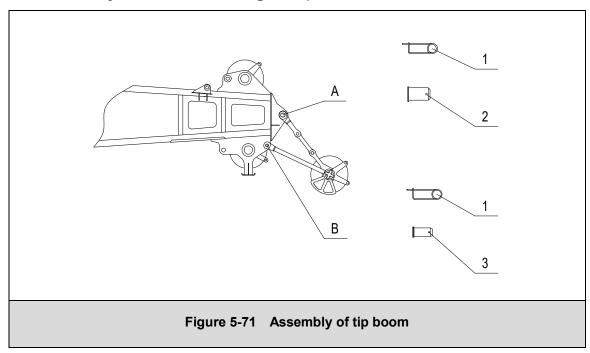
The procedures for assembly of tip boom are shown in figure 5-71:
