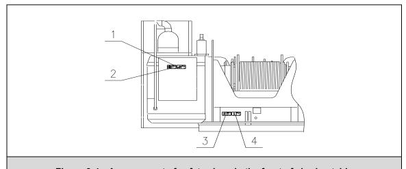
Figure 3-4 Arrangement of safety signs in the front of slewing table
