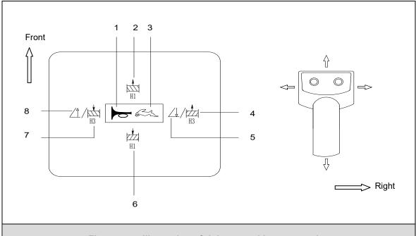
Figure 4-4 Illustration of right control lever operation
