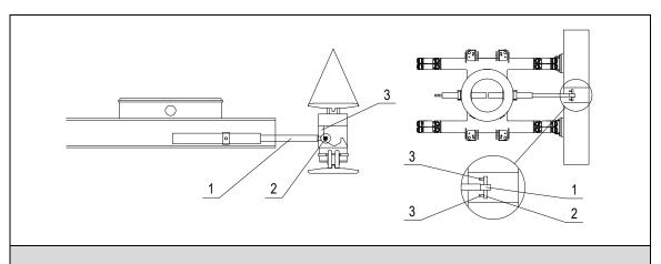
Figure 5-11 Assembling crawler carrier with the help of horizontal cylinder
