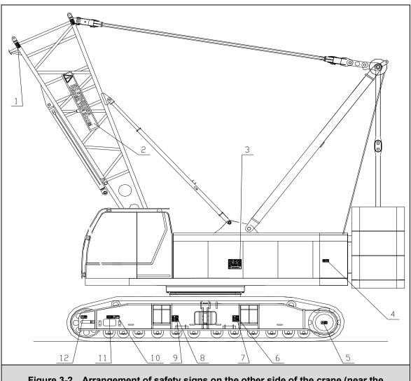
Figure 3-2 Arrangement of safety signs on the other side of the crane (near the operator's cab)
