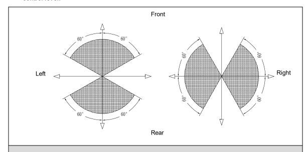
Figure 4-36 Valid area of control lever when operating a single movement
