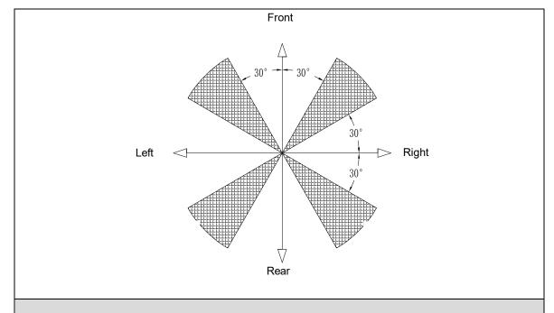
Figure 4-37 Valid area of control lever when operating a simultaneous movement
