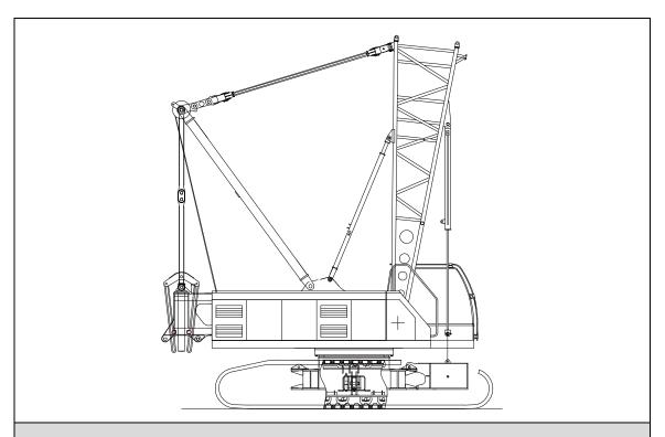
Figure 5-26 Attachment of central counterweight on the undercarriage central section
