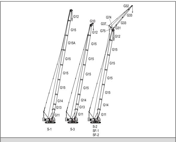
Figure 5-37 Available boom configurations
