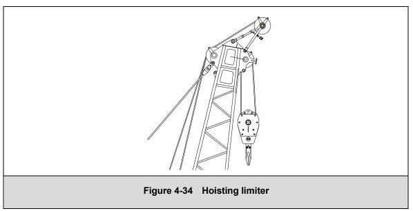
The hoisting limiter is installed to prevent the hook pulley from colliding with the boom head. Before using the crane every time, inspect the switch by lifting the hook to the upper limit and colliding with the hoisting limit switch weight.
