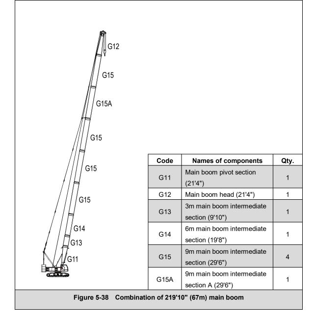
When different length of main boom is required, crane operator only needs to disconnect main boom pivot section from main boom head, and then install main boom intermediate sections between them. In this way, main boom can be assembled to required length. The assembly of main boom from 42'8" (13m) to 219'10" (67m) is shown in the table 5-8.
