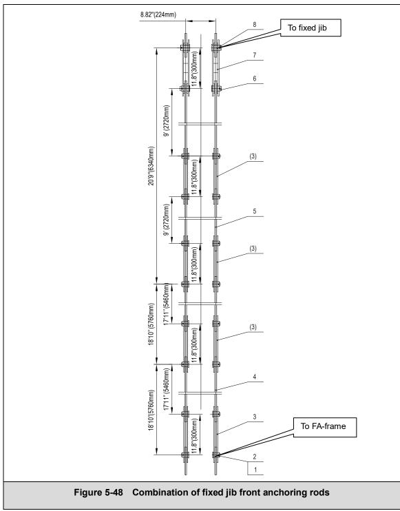
The explanation of component numbers in the figure 5-48 is shown in the table 5-12.
