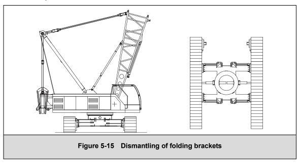
a) Retract support cylinders, put support plates on the attachment points at the side of folding brackets, disconnect hydraulic connection of folding brackets and tilt support cylinder. See the figure 5-16.
