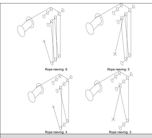
Figure 4-51 Reeving 55USt (50t) load hook
