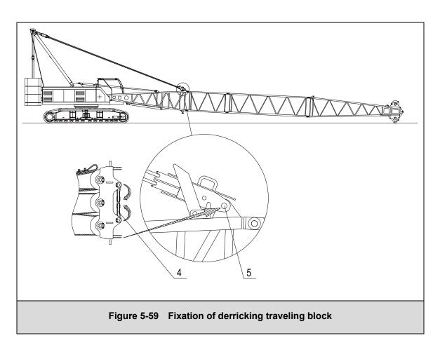
Table 5-15 Fixation of derricking traveling block
