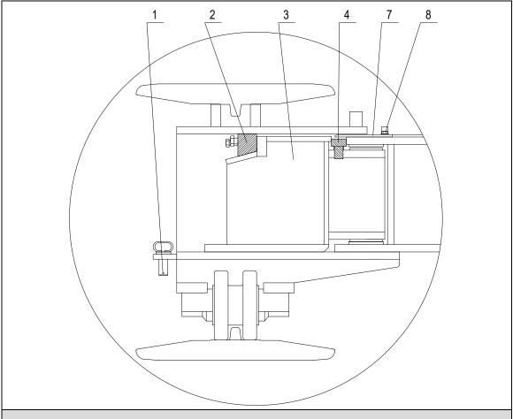
Figure 5-18 Enlarged view of crawler carrier extending & retracting mechanism
