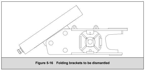
b) Dismantle folding brackets by use of mounting cylinder or other device, and then connect the horizontal anchoring rods.
