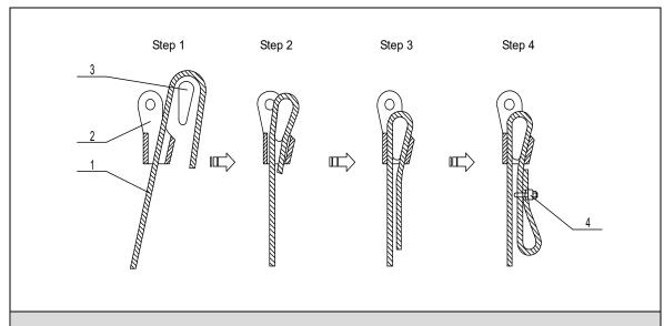
Figure 4-59 Fixation of rope end point
