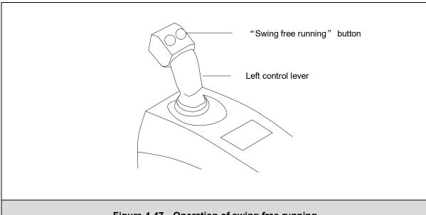
Figure 4-47 Operation of swing free running
