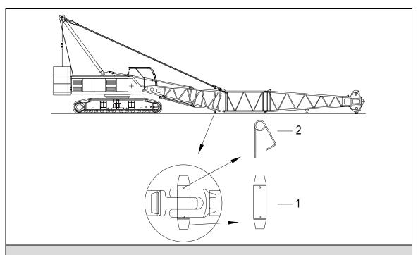
Figure 5-53 Bolt preassembled main boom sections to main boom pivot section
