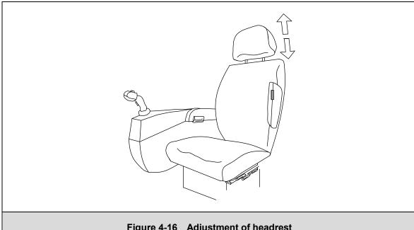
Figure 4-16 Adjustment of headrest
