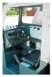
Standard: Open air cab shell with overhead safety glass Optional: Closed cab with hinged door, heater/ defroster, and all window glass
