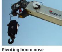
Standard on the YB4409-2 and YB4411 the exclusive pivoting boom nose allows operators to decrease the overall boom head depth and operate in more confined areas.
