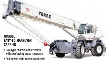
• rull power-shift transmission with integral torque converter; neutral safety start; 6 speeds forward 3 reverse.
