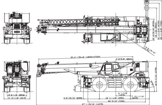
Note : Dimension is with boom angle at -1.5 degree.
