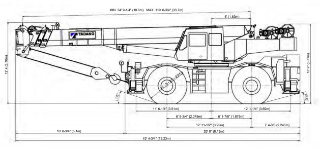
Note: Dimension is with boom angle at -1.5 degree.
