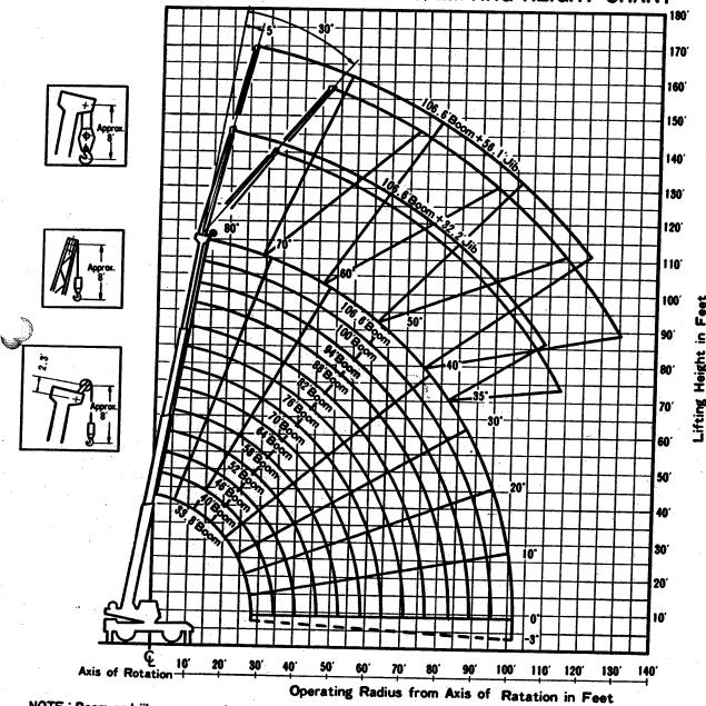
NOTE: Boom and jib geometry shown are for unloaded condition and machine standing level on firm supporting surface. Boom deflection and subsequent radius and boom angle change must be accounted for when applying
