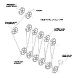
THIS CHART IS ONLY A GUIDE WID SHOULD NOT BE USED TO OPERATE THE CRAME. The individual crame's load chart, operating instructions and other instructional plates must be read and understood prior to operating the crame.
