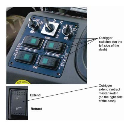
Figure 07 – 4 Outrigger Switches
