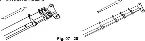
c) After the boom extends to required position, slowly tilt the pedal backward to neutral position;
