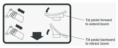
Figure 06 - 8 Boom Extend / Retract Pedal
