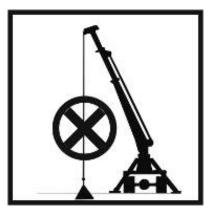
(9) Do not extend / retract the boom with a suspended load.
