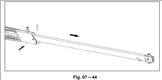
k) Reeve the auxiliary hoist rope. Install the auxiliary hook and the anti-two block switch. Check the jib for proper assembling.
