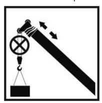
(10) Keep no less than 3 wraps of wire rope on the drum.
