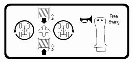
Figure 06 – 7 Left Joystick (Swing / Aux. Winch Control)
