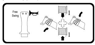
Figure 06 – 10 Right Joystick (Boom Hoist / Main Winch Control)
