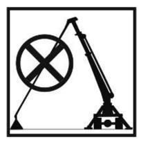
(8) Do not try to lift a load that is buried or frozen on the ground.
