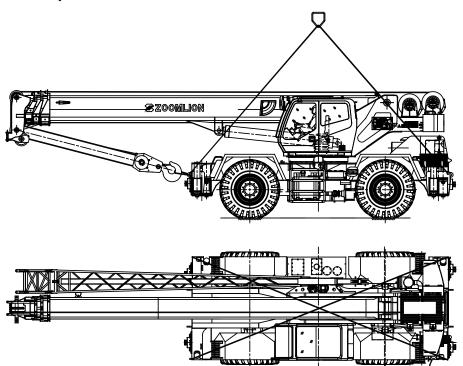
Figure 08 – 1 Crane Lift Points
