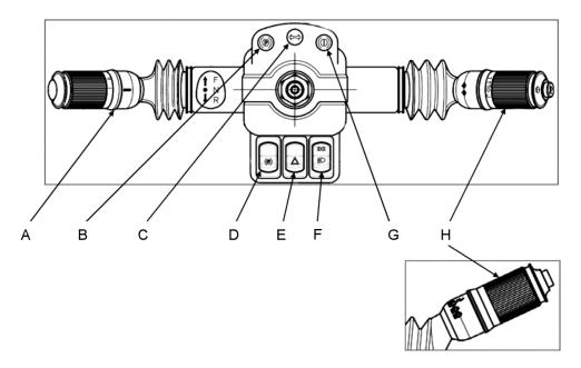
Figure 06 – 9 Combination Switches
