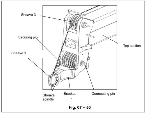
Use of this rooster sheave saves the time of hoist when lifting small load ( $\leq$  5.5 Ton) with auxiliary hook, thus to improve the working efficiency.
