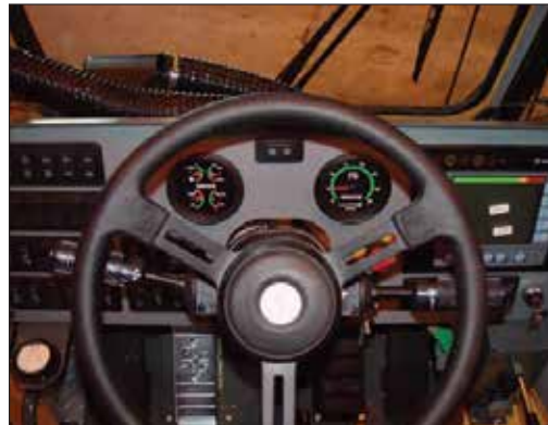
Automotive-style dash control panel designed to offer a less cluttered look while still offering full instrumentation.
