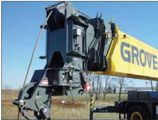
The RT540E incorporates a rectangular boom shape made from 100k.s.i. steel which eliminates weight and maximizes structural capacities.
