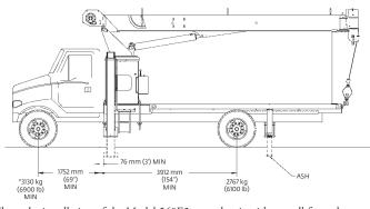
Allows the installation of the Model 560E2 on a chassis with a small frame by using the standard sub-base for 18 ft bed. In most cases, the chassis will not require reinforcing, and the amount of counterweight required is minimized, increasing payload capacities.
