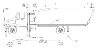
Requires front SFO stabilizer to give machine full capacity 360° around the truck. Truck must meet the minimum requirements above. Front stabilizer gives the machine a solid base, helping the operator control loads precisely.
