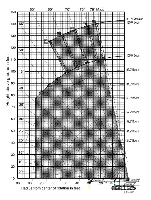
Limits of operation: Maximum load capacity = 750 lb Maximum radius when mounted on main boom = 75 ft Minimum boom angle when mounted on 30 ft extension = 60°
