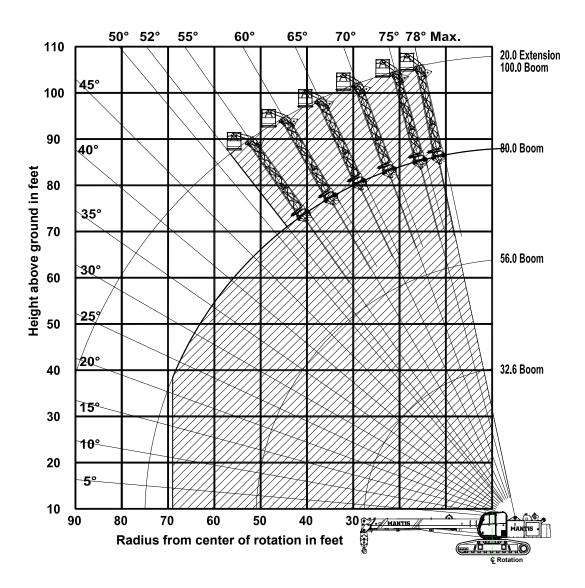
Shaded Area is Allowable Operating Range Limits of operation: Maximum load capacity = 750 lb Maximum radius when mounted on main boom = 69 ft Minimum boom angle when mounted on 30 ft extension = 52°
