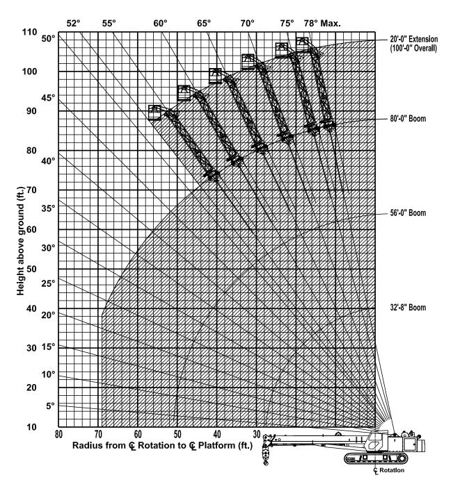
Limits of operation: Maximum load capacity = 750 lb Maximum ra
