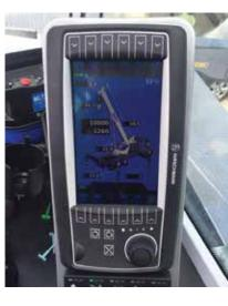
Externally routed A2B cable. LMI with crane function cut-offs for overload protection. Color graphic display, event recorder, WADS-Work Definition System.
