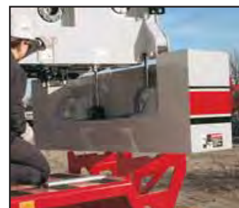
Fast & efficient hydraulic counterweight removal enhances roadability
