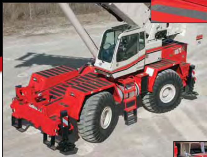
Fast & efficient hydraulic counterweight removal enhances roadability
