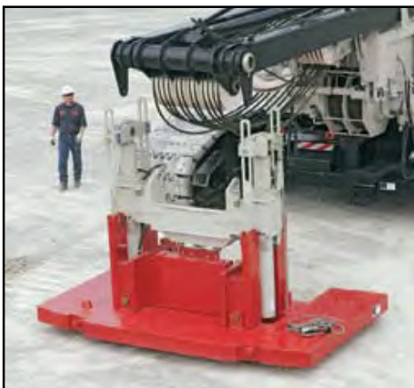
Counterweight removal mechanism detached
