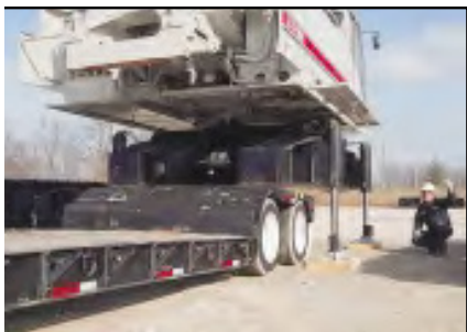
Hydraulic jacking system lifts the upper, lower frame and treadmembers off the ground. Treadmembers are removed and a trailer can then be backed under the lower frame and upper for transport.
