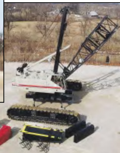
Optional 10' (3.05 m) boom extension handles treadmembers, counterweight and boom during self-stripdown or erection.
