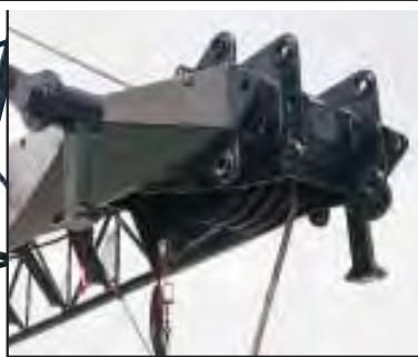
*The boom top section features **standard pin-on points** for adding optional attachments such as a fixed jib, tip extension and adapters for universal pile driving leads.*
