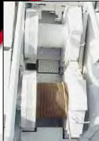
Load hoist drums contain a pilot-controlled bi-directional axial piston motor and a planetary gear-reduction unit to provide positive control under all load conditions.
