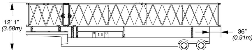
**LOAD #4 – 36,326 lb (16 477kg)**Lower counterweight, 40 ft (12.19m) boom extension,
