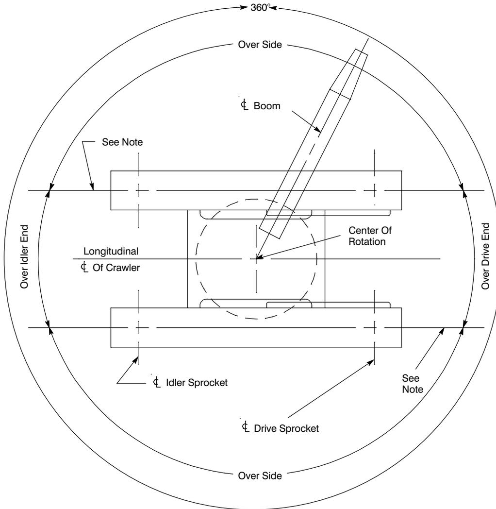
**Note:** These Lines Determine The Limiting Position Of Any Load For Operation Within Working Areas Indicated.
