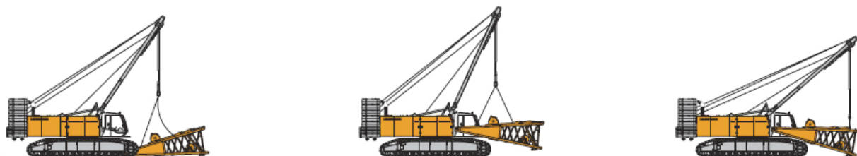
Unloading and assembly of main boom foot
