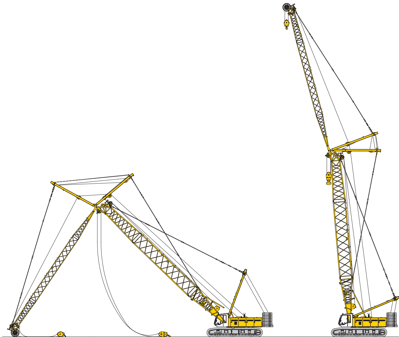
Erecting of main boom and luffing jib
