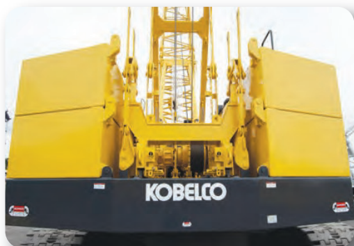
Self Lifting Device - Standard Equipment
