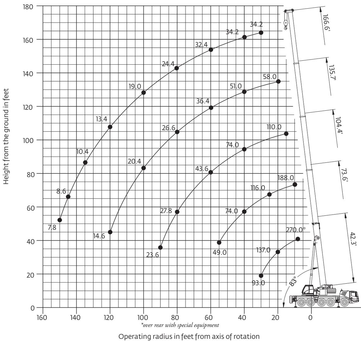
Hook heights shown in the working range diagram do not consider loaded boom deflection.
