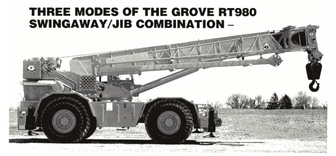
The 32 ft. Swingaway and optional 28 ft. A-frame jib can provide the RT980 with an additional 60 ft. of reach capability, conveniently stowed on the crane. The three different modes of this combination are:
