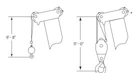
Dimensions are for largest Grove furnished hook block and headache ball, with anti-two block activated.
