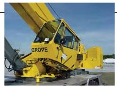
The "E" Series cab on the RT9130E tilts up to 20° providing the operator additional comfort when working at long boom and extension lengths.
