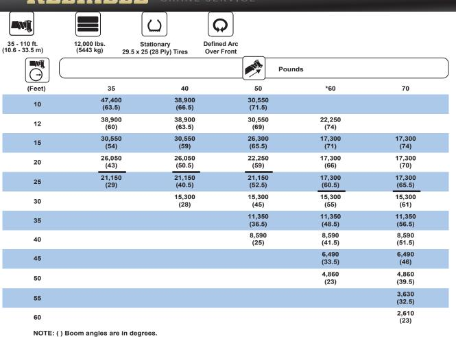
\*60 ft. boom length is with inner-mid extended and outer-mid & fly retracted.
