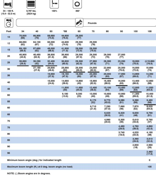
\*58 ft. boom length is with inner-mid extended and outer-mid & fly retracted.
