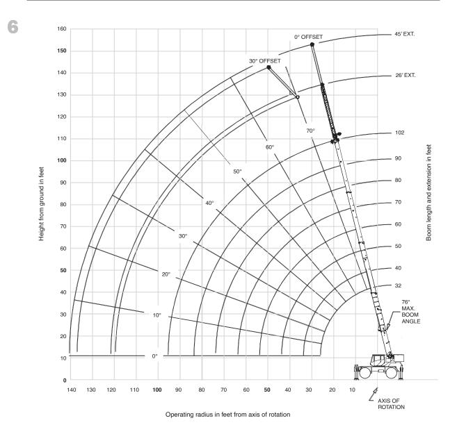
Dimensions are for largest Grove furnished hook block and headache ball, with anti-two block activated.
