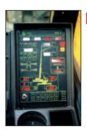
EKS4 is an electronic load moment indicator that operates in conjunction with ECOS continuously displaying crane configuration and load moment data
