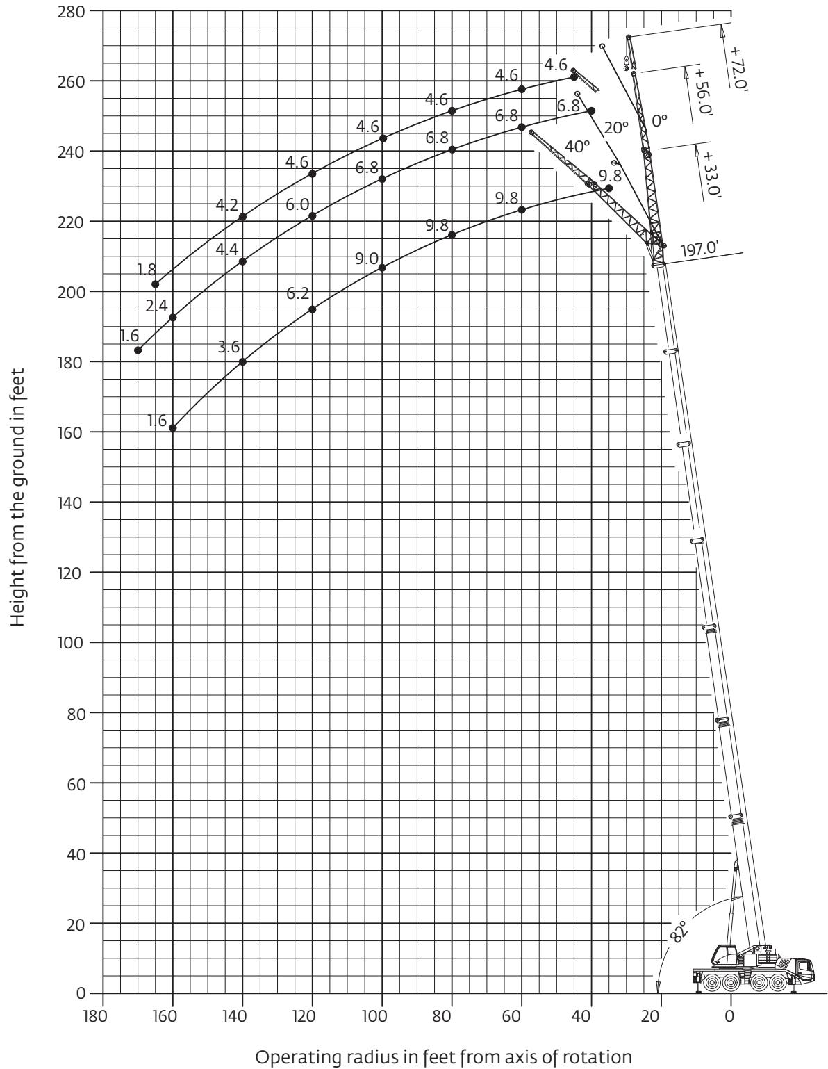
*Hook heights shown in the working range diagram do not consider loaded boom deflection.*
