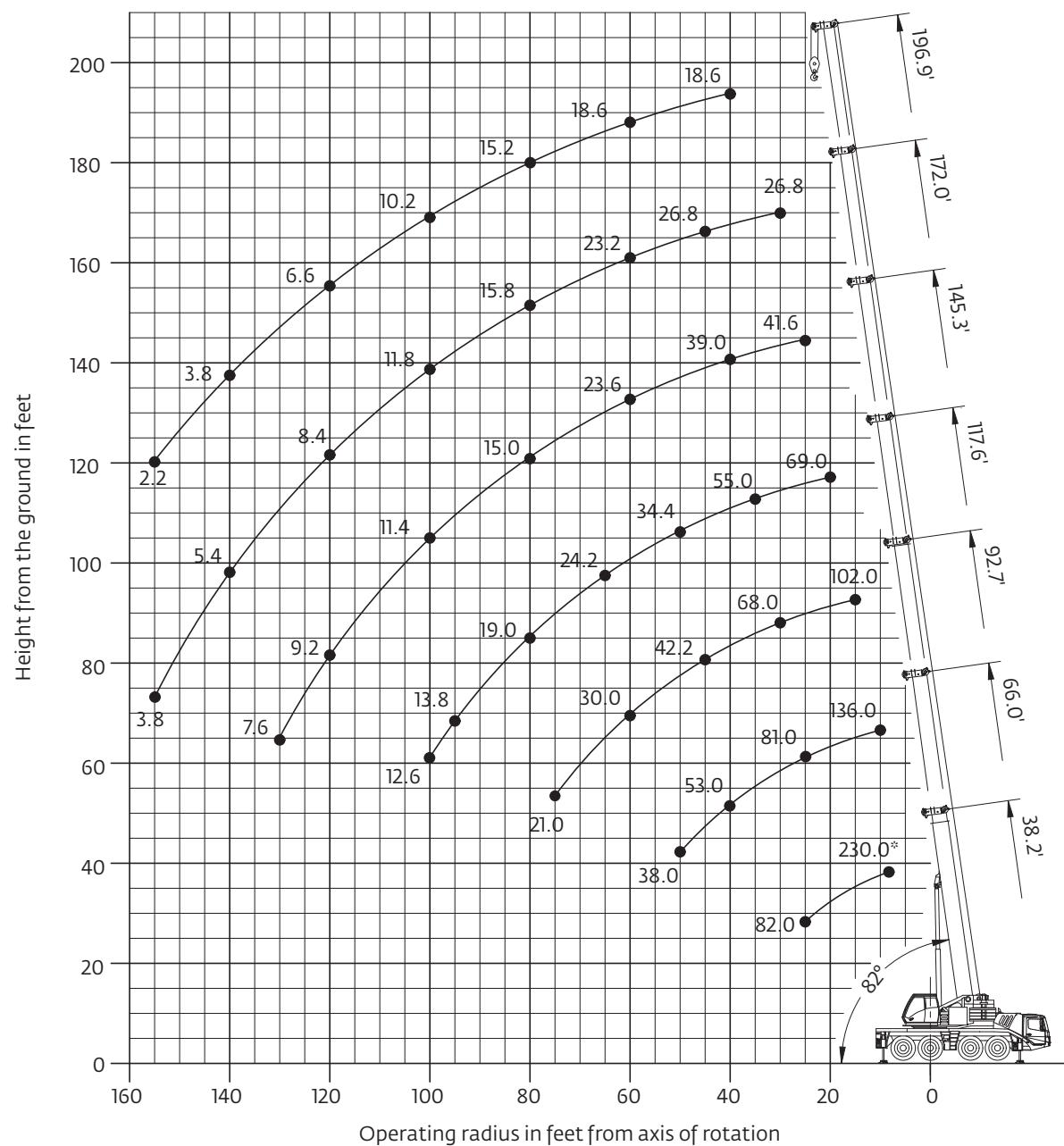
*Hook heights shown in the working range diagram do not consider loaded boom deflection.*
