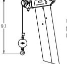
Dimensions are for the largest Grove furnished hook block and overhaul ball, with anti-two block activated.
