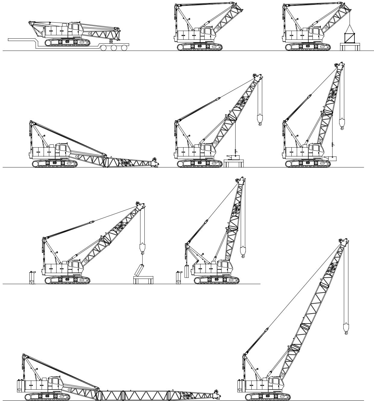
**CK850-III Counterweight Self-Removal Device
