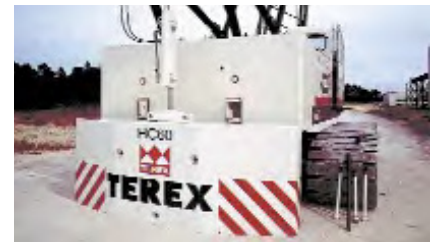
Hydraulic removable counterweight system
