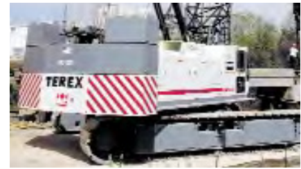
Counterweight hydraulically extends
