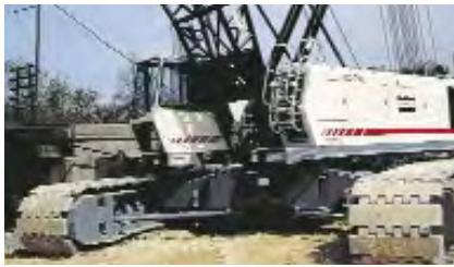
Extra wide cab is set forward of boom foot
