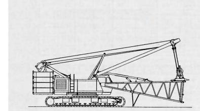
The mast is used to lay out boom sections and install the boom butt. Power-activated pins simplify installation of the butt.
