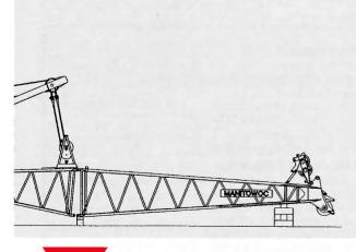
Boom inserts and top are pinned to the boom butt. Boom-support pendants are pinned to the mast and boom top. Main and auxiliary load lines are reeved.
