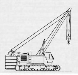
The gantry is lowered and pinned to the assembled counterweight. Hydraulic cylinders raise the gantry and counterweight to working position. The counterweight is then connected to the back of the upperworks by
