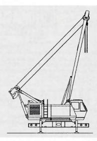
Hydraulic cylinders raise the gantry to working position and lift the mast to vertical. The boom hoist rigging then lowers the mast so it can be rigged with the set-up load block. Wire rope from one of the hoist drums is reeved through sheaves in the mast to rig the block.
