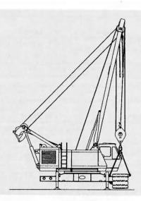
The mast is used to install the crawlers, handle boom sections, stack the counterweights, and lift other components. Crawlers attach using FACT alignment surfaces and powered pins.
