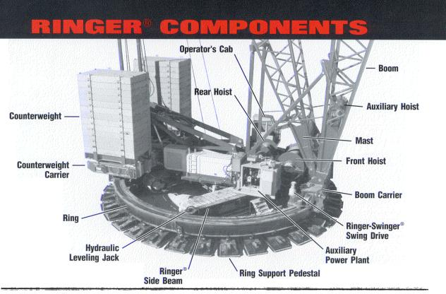
Ringer® Side Beams: High-strength beams connect ring to basic crane. FACT™ connectors simplify set-up. Beams provide mounting for four hydraulic jacks that level the ring during set-up.
